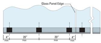
System for 200 lb. point load with 2 × safety factor 20" center-to-center maximum with 4" maximum from center to glass edge.
