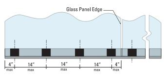
System for 200 lb. point load with 4 × safety factor 14" center-to-center maximum with 4" maximum from center to glass edge.
