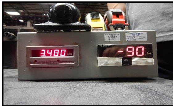
Residual Deflection at 90 lbsf Actual Deflection of 0.029 in
