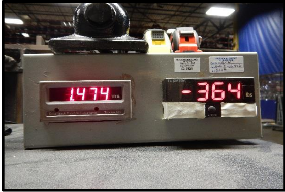
Ultimate Test Load of 365 lbsf Actual Deflection of 2.145 in
