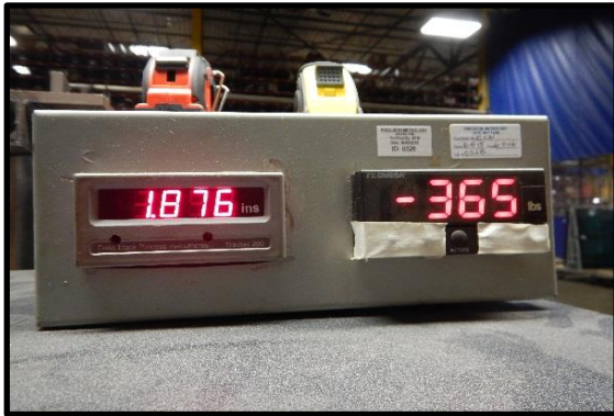
Ultimate Test Load of 365 lbsf Actual Deflection of 1.709 in
