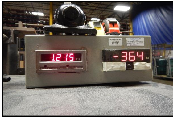
Ultimate Test Load of 365 lbsf Actual Deflection of 2.299 in
