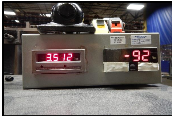
Residual Deflection at 90 lbsf Actual Deflection of 0.073 in
