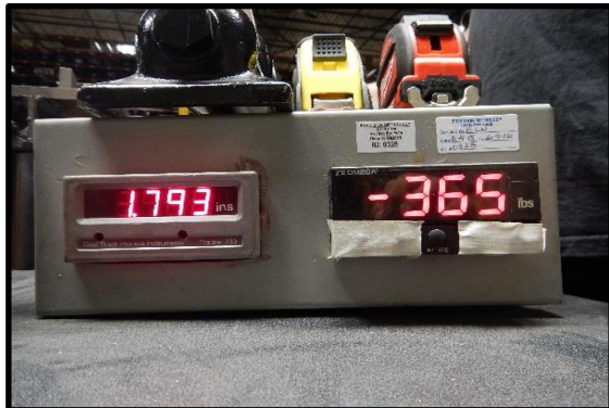
Ultimate Test Load of 365 lbsf Actual Deflection of 1.785 in
