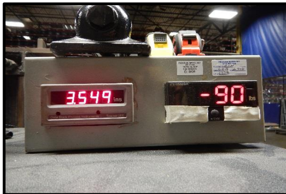
Residual Deflection at 90 lbsf Actual Deflection of 0.07 in
