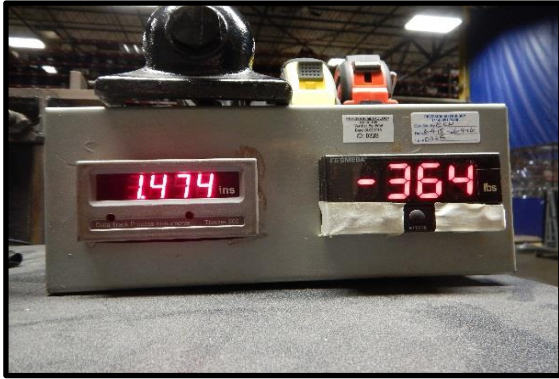
Ultimate Test Load of 365 lbsf Actual Deflection of 2.12 in
