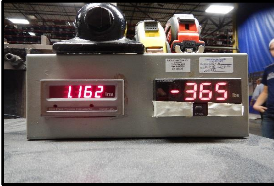
Ultimate Test Load of 365 lbsf Actual Deflection of 2.347 in
