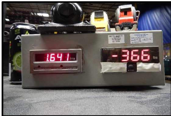
Ultimate Test Load of 365 lbsf Actual Deflection of 2.322 in
