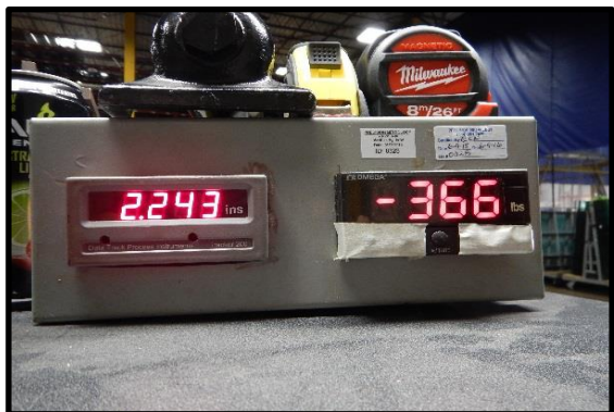
Ultimate Test Load of 365 lbsf Actual Deflection of 1.743 in
