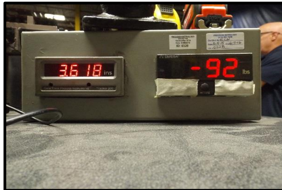
Residual Deflection at 90 lbsf Actual Deflection of 0.013 in
