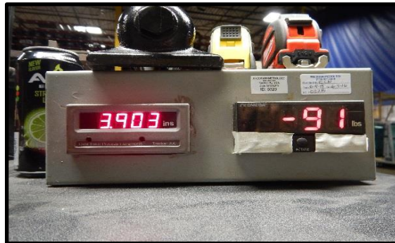
Residual Deflection at 90 lbsf Actual Deflection of -0.015 in
