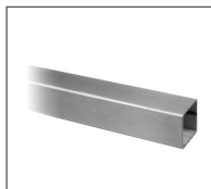
SQUARE POST (2) 1.57" x 1.57" POSTS 40" LONG .078" WALL THICKNESS, PREDRILLED 304 Stainless Steel #4 Brushed Finish Part #: R13-4900-040-12
